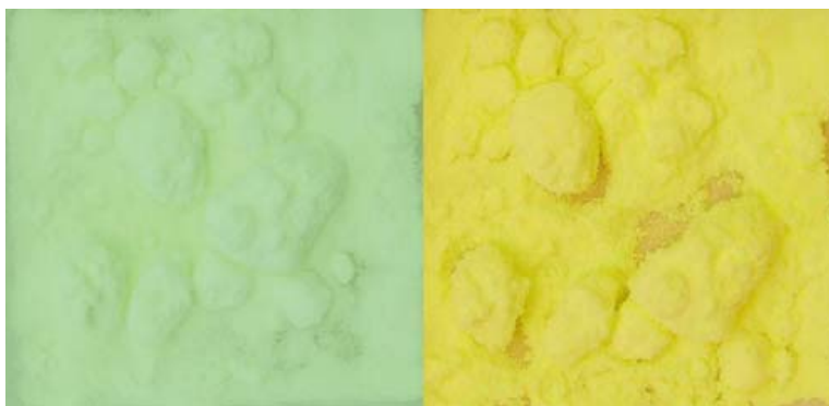
Figure 2 Contrast in the color of elemental sulfur immediately after removal from liquid nitrogen temperatures (left) and after warming to ambient (right).
